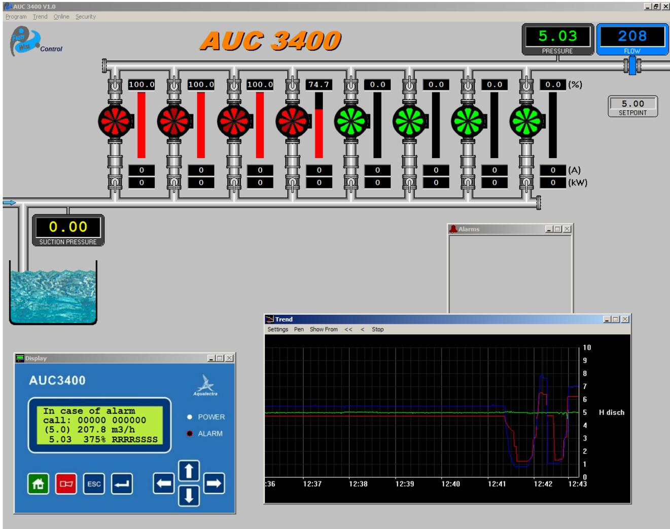
Connecting a PC running the AUC3400.exe Windows program on the serial port, either by a local direct connection or remotely through a modem dial up connection offers interesting benefits.
