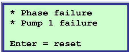
In this case there is a pump failure and a phase failure.
