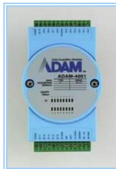
The ADAM modules are controlled over the RS485 communication line.
