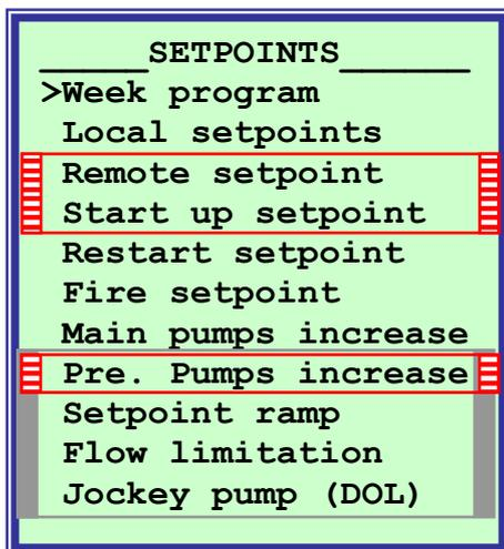
The core of the setpoint program is a week program. This is a sophisticated time clock that you can program to run all kinds of jobs, including different setpoints, test runs and pump changes.
