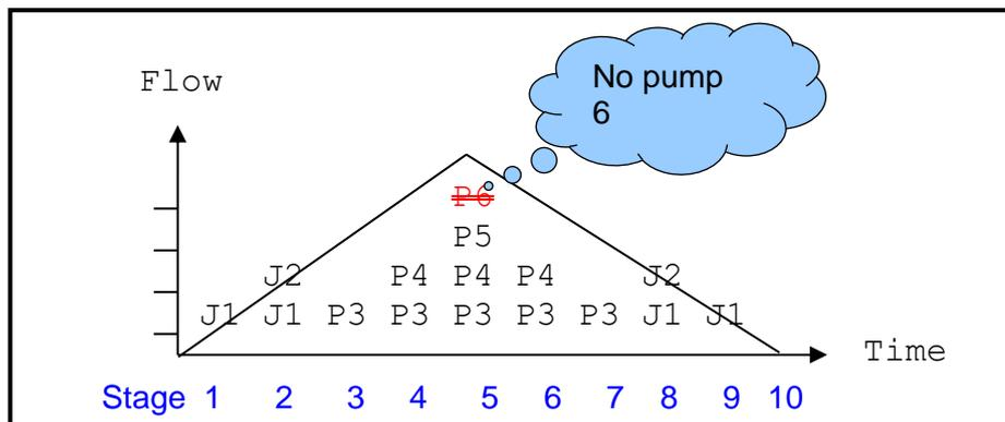
As the flow increases upward from zero the following happens in each stage:
