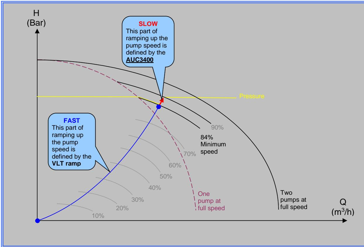
The figure shows what happens when one pump operates at maximum speed and the flow demand increases. The pressure will drop and the AUC3400 will start the second pump. The second pump ramps up to minimum speed following the FC ramp setting (fast). Then, at minimum speed, the pump ramps up following the AUC3400 ramp (slow).
