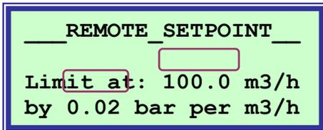
If flow limitation is enabled, you can also define how the setpoint ramps down as the flow increases above a set value. In this example the setpoint of 5 bar will ramp down by 0,02 bar per m<sup>3</sup>/h when the flow passes 100 m<sup>3</sup>/h. At 150 m<sup>3</sup>/h the setpoint will be limited to:
