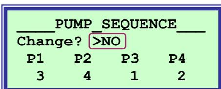
The pump sequence is the order in which pumps are started and stopped.
