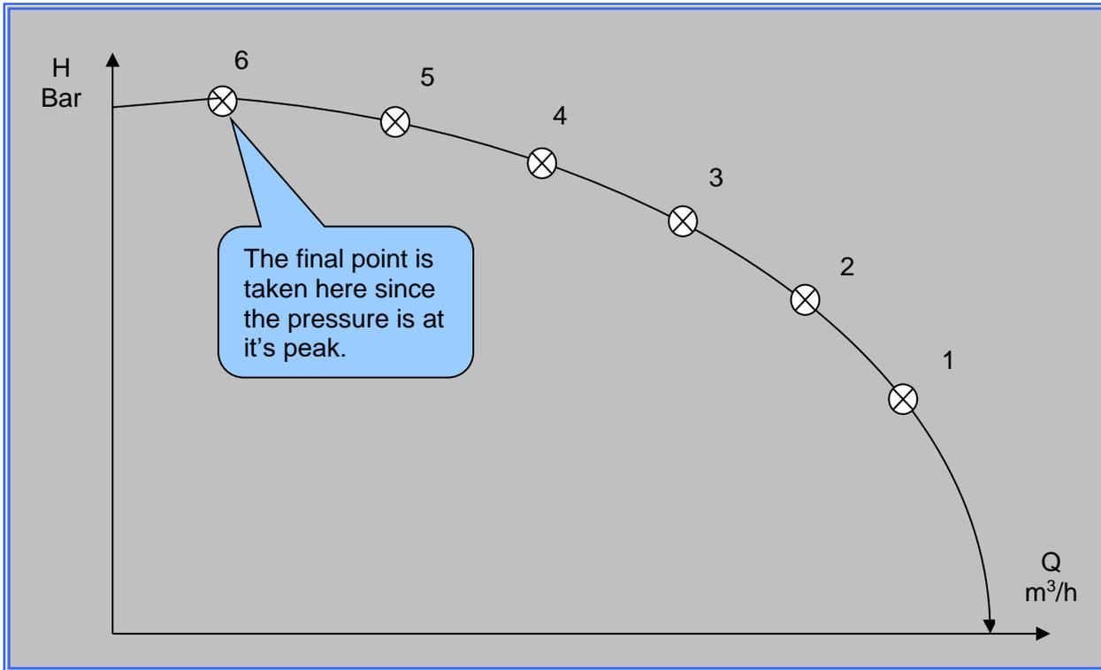
The above figure show what the sequence of recorded point is. They also show the point are taken at equal distance and that the last point should be taken at the highest pressure value, not necessarily zero flow.
