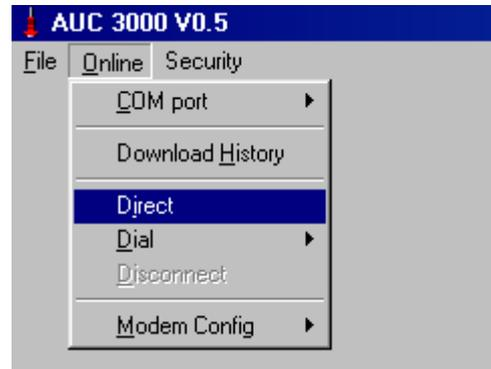
To set up a remote modem connection you need to initialise the modem first, therefore select:
