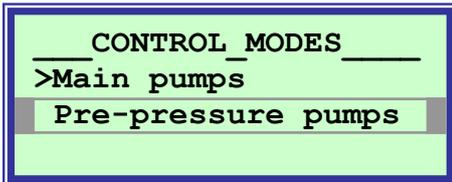
In the pump sequence menus, you control the way pumps are changed over.
