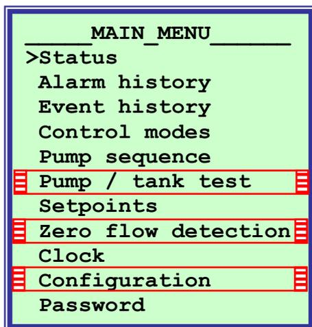
Use the UP and DOWN arrow keys to scroll up or down and press enter or RIGHT arrow to select an option. The current option being considered below is indicated by the “>” sign.
