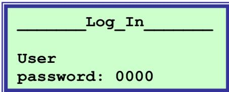
The display asks for a user password. The user password or service password are both accepted by the AUC3400. If you enter the user password the display shows:
