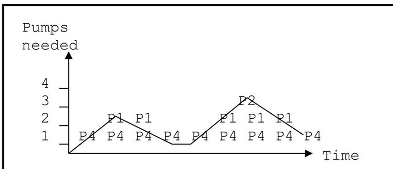
So the pump sequence does not alternate by the starting and stopping of the pumps. It remains fixed until a pump change is instigated either manually by means of the above display or automatically by the week program. In the week program you can program a pump change at any time of the week (even on a daily basis, refer to section 15.7.1).
