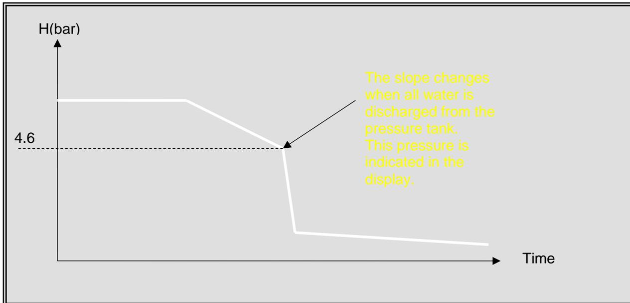
Once the air pressure in the diaphragm tank is determined by the AUC3400, you may get an alarm, now or in the future, that the air pressure in the tank is too low or too high in relation to any of the setpoint values that have been specified.
